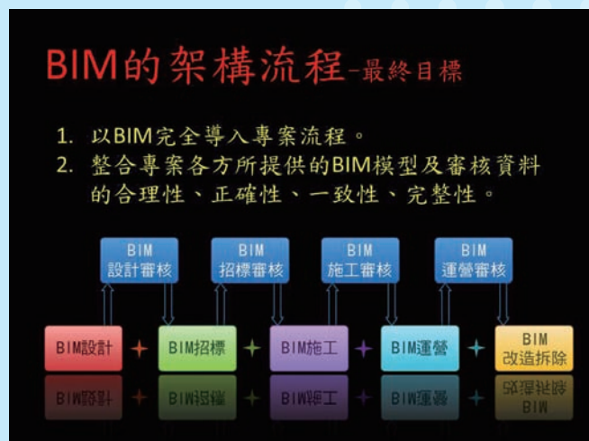
BIM 的架構流程 Structure/Flowchart of BIM System
